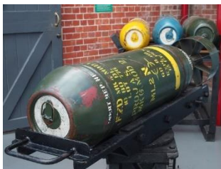
Anti-Submarine (AS) Mortar Length 150 cm Diameter 305 mm
